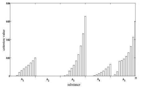
Pic. 4. The sensitivity of reagent and product concentrations of phthalic anhydride to kinetic parameters *k*<sub>3</sub>.
