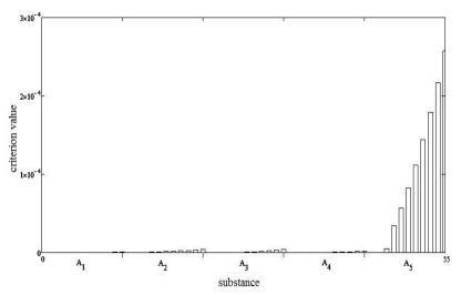
Pic. 7. The sensitivity of reagent and product concentrations of phthalic anhydride to kinetic parameters *k*<sub>6</sub>.
