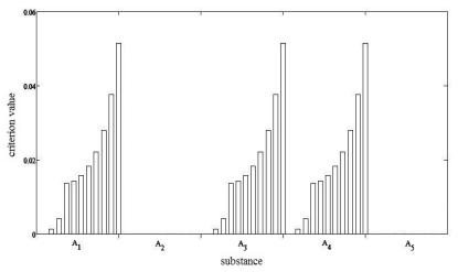
Pic. 2. The sensitivity of reagent and product concentrations of phthalic anhydride to kinetic parameters *k*<sub>1</sub>.
