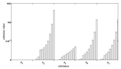
Pic. 3. The sensitivity of reagent and product concentrations of phthalic anhydride to kinetic parameters *k*<sub>2</sub>.
