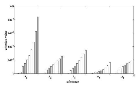
Pic. 5. The sensitivity of reagent and product concentrations of phthalic anhydride to kinetic parameters *k*<sub>4</sub>.
