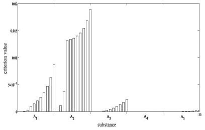
Pic. 6. The sensitivity of reagent and product concentrations of phthalic anhydride to kinetic parameters *k*<sub>5</sub>.
