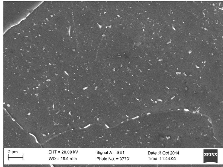
**Figure 2.** Microstructure of the in-service aged material with heat treatment condition (ISAM+HT)
