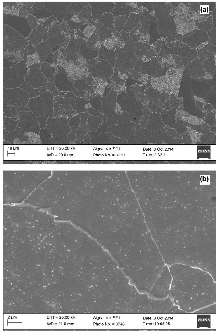
**Figure 1.** (a) Ferritic-perlitic microstructure of the in-service aged material (ISAM) condition; (b) Intragranular and intergranular precipitation in the in-service aged material (ISAM) condition.
