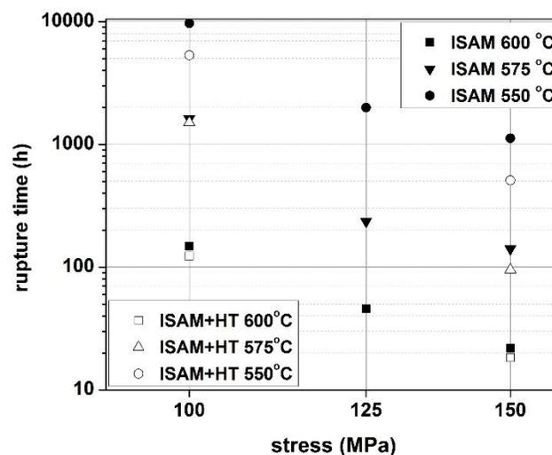
**Figure 5.** Creep rupture time of ISAM (in-service aged material) and ISAM+HT (in-service aged material and subjected to heat treatment) conditions, for different test combinations of stress and temperature.
