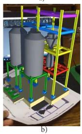
Figure 3. a) Mechanical structure drawing that serves as a marker. b) AR display through the Scope<sup>®</sup> app.
