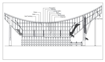
Figure 4. Structure and Construction of one of Mamasa's tarditional house types
