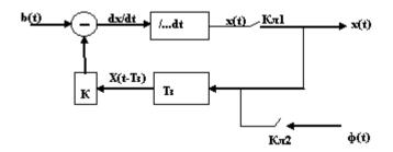
Fig.1. Block diagram of the model with memory
