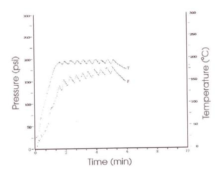
Figure 1. Monitoring temperature and pressure in closed reactors heated by microwave irradiation in the MDS-2100 microwave oven.
